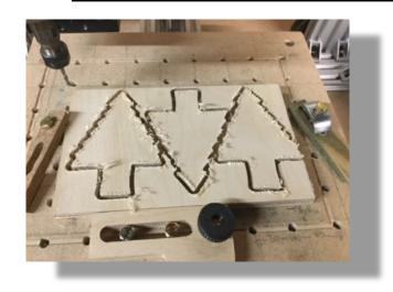
Requested to produce 600 wooden Christmas trees for an event. Using a members CNC cutter machine the project was able to produce three trees on one small sheet of plywood.
